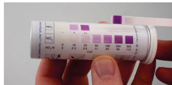
Figure 5. Comparing the colour on the strip with the scale on the test strip bottle. The recommended product is from Merck (MQuant® 0 – 500 ppm strips).
