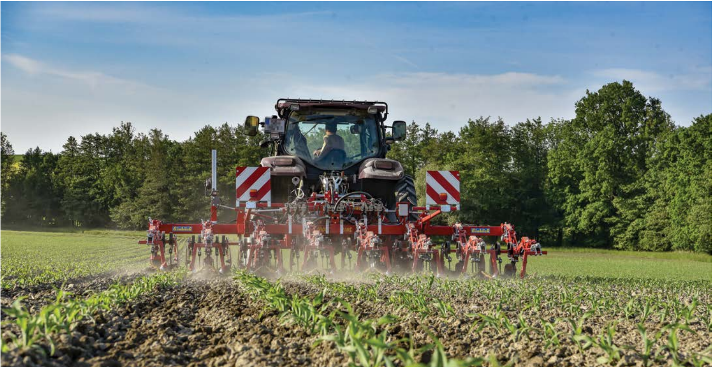
Austrian manufacturer Einböck's CHOPSTAR row hoe equipped with the automatic camera steering system ROW-GUARD
