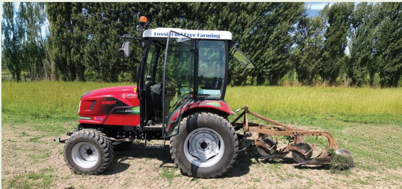
The Energy Farm's new compact electric 55hp Knecht 404G2E - an acquisition made possible by the Energy Efficiency and Conservation Authority (EECA) Demonstration Fund, Meridian Energy and Power Turf New Zealand
