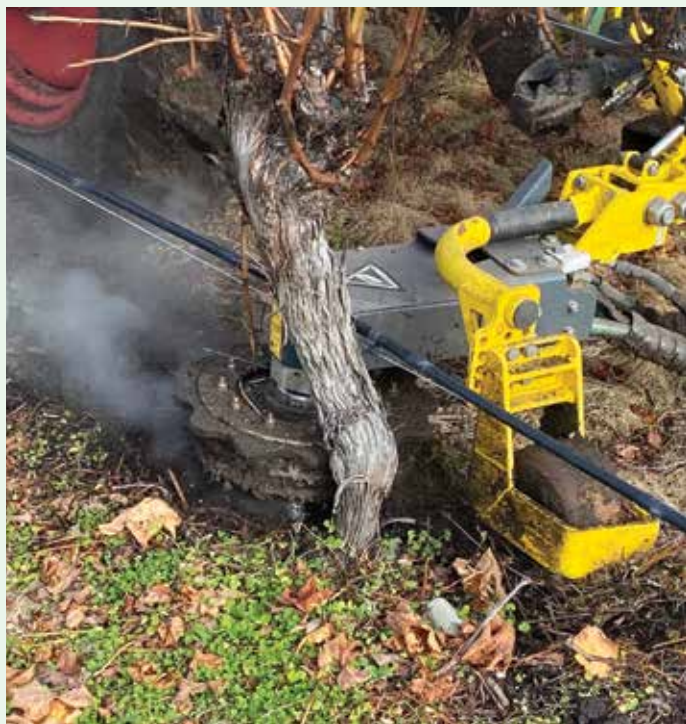
Figure 2: The high-pressure waterjet weeder operating - the treated area can be seen to the left of the steel post
