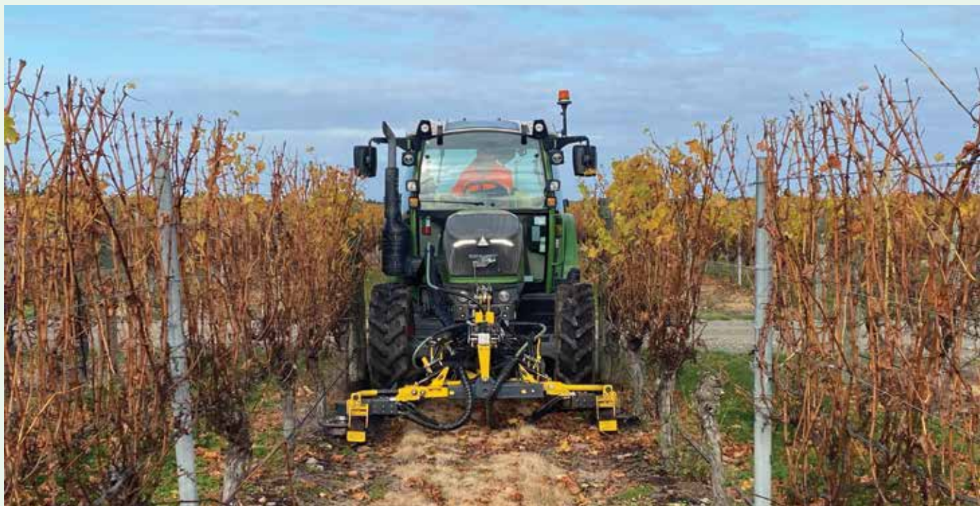
Figure 1: A high-pressure waterjet weeder operating in Waiata Vineyard, Waipara, Canterbury
