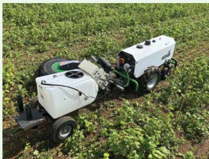
GOVOR is a lightweight electric tractor designed to automate outdoor manual labour tasks for row-based growers
