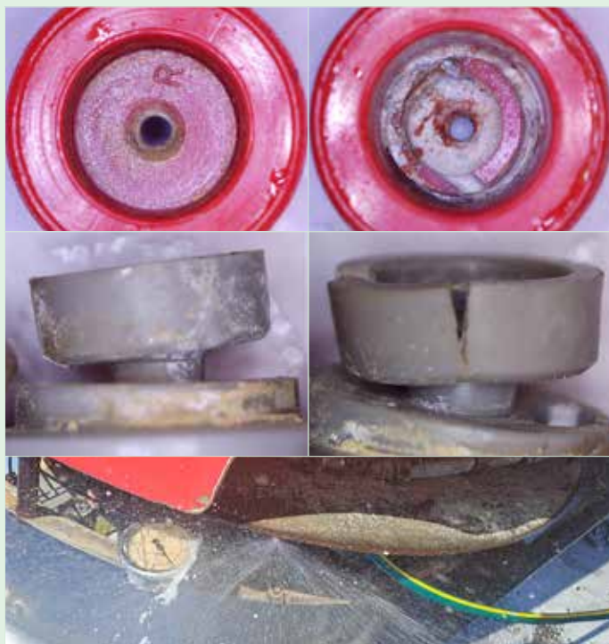
Defects found with nozzles during annual sprayer calibration. Damaged or defective nozzles negatively impact spray output quality and amount
