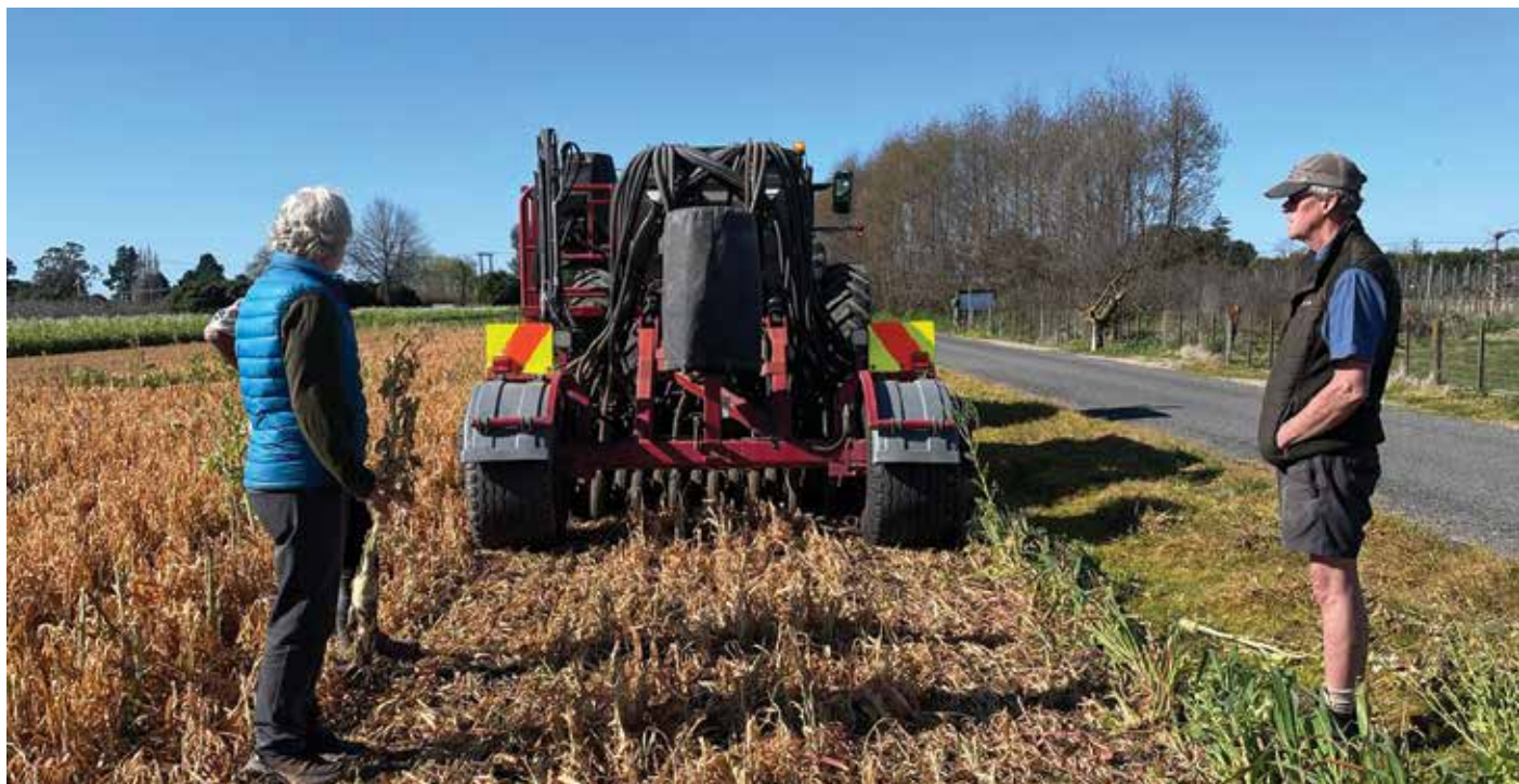
Doing a test run with Mike Kettle's Allen direct drill, planting peas into sprayed out cover crop in the 'hybrid' treatment
