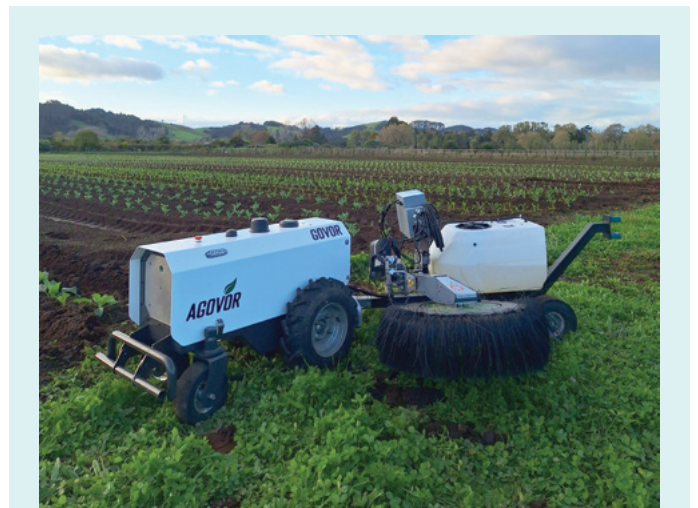
In 2020, Agovor founder and nurseryman Richard Beaumont partnered with Simon Carroll, a seasoned automation engineer, to develop GOVOR, an autonomous mini tractor that could fit between his tree rows. One or more GOVORs can be managed from a phone or computer, using AI technology to navigate autonomously, and whatever attachments are needed to complete the task required
