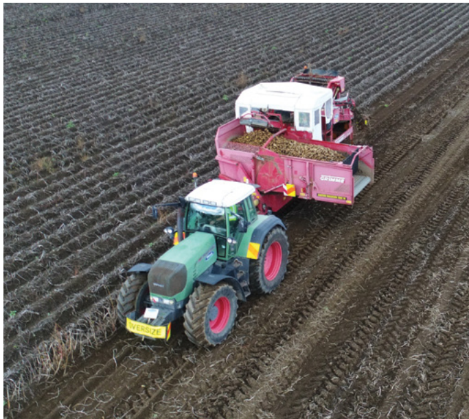
Figure 1: One of the two Grimme potato harvesters fitted with Greentronics yield monitors, harvesting one of the trial sites
