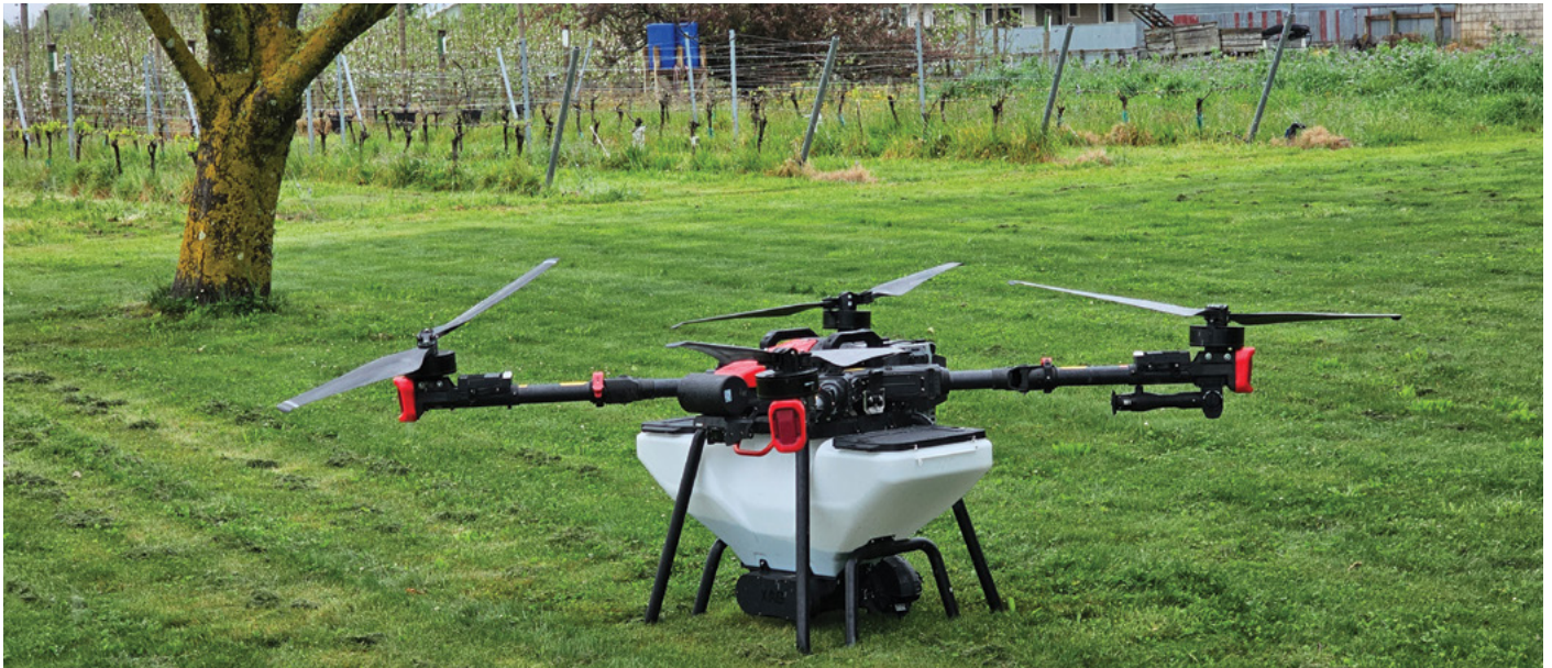
Airborne Solutions demonstrated using large quadcopters for spraying. LandWISE contracted them to apply slug bait and nutrient products to trial plots at the MicroFarm
