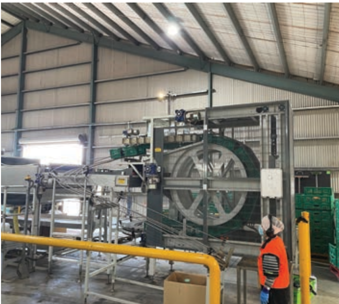
A bespoke auto infeed to empty full produce crates onto a packing line
